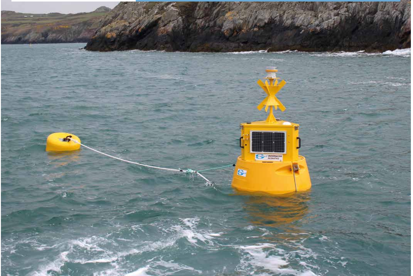
Buoy for automatic and real-time detection of cetaceans, deployed in Wales in 2023
