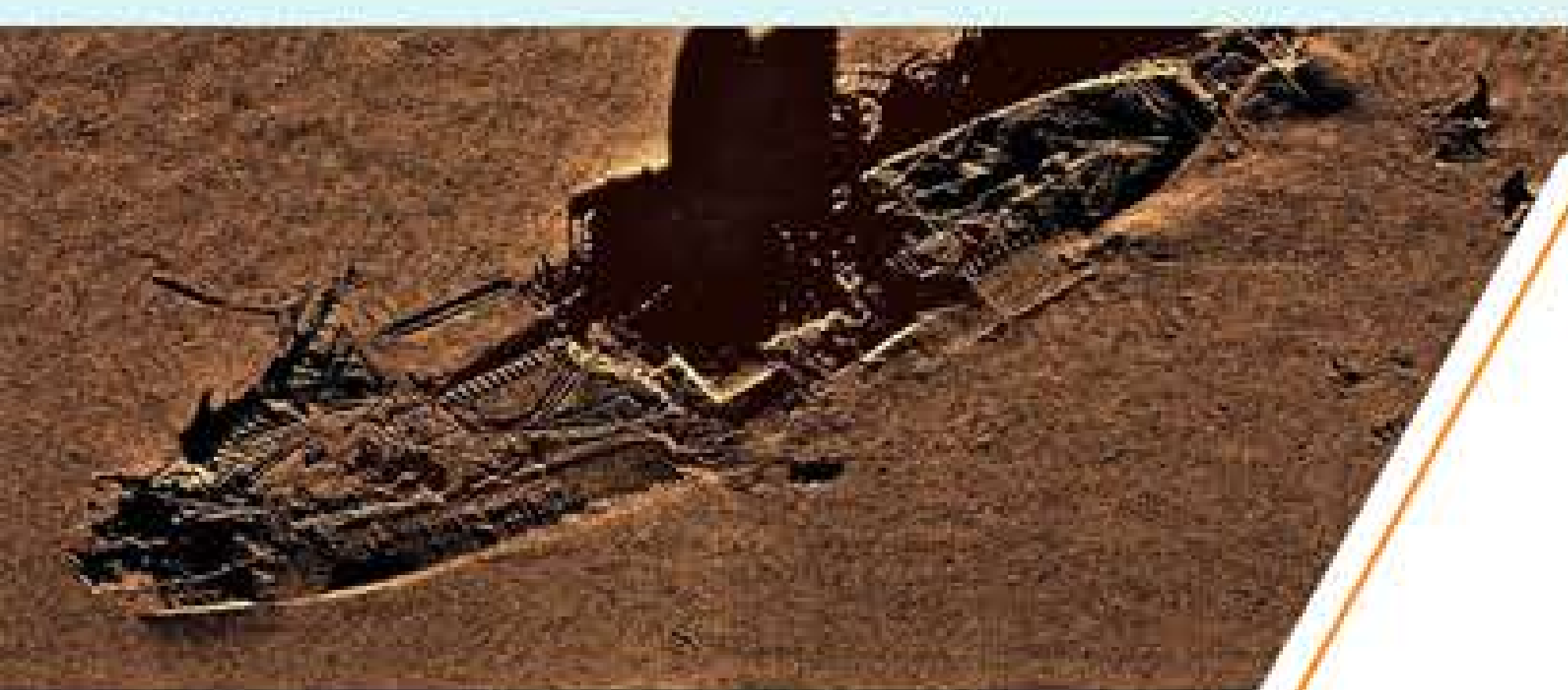
High resolution picture of wreck obtained by synthetic aperture sonar ©THALES
